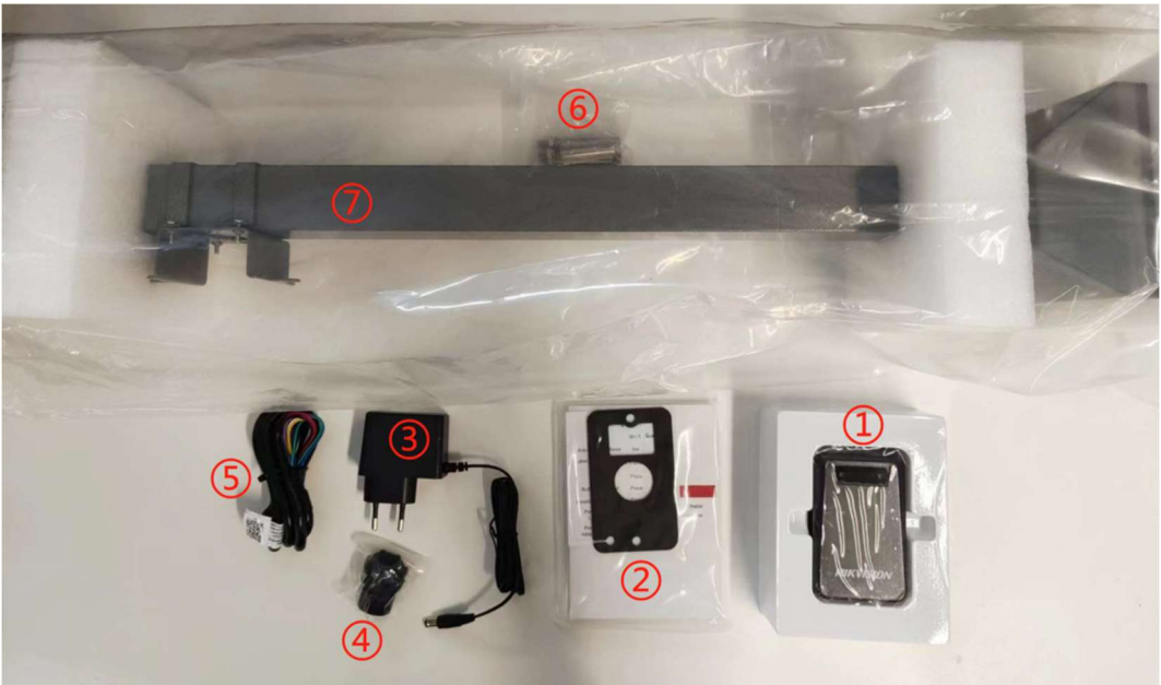
① Radar ② User Manual ③ Power Cable ④ Nut ⑤ Signal Line ⑥ Expansion Screw ⑦ Pole
