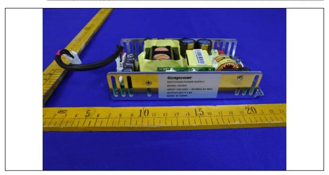
Details of: Built-in power supply (P1A-F10250-D-S1)
