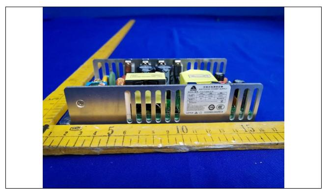
Details of: Built-in power supply (P1A-F10250-D-S1)
