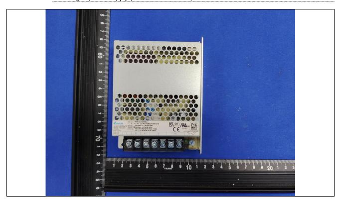
Details of: Building-in power supply LRS-100-12
