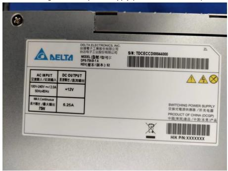
Marking for Alternative built-in power supply (model SFXA1071A)
