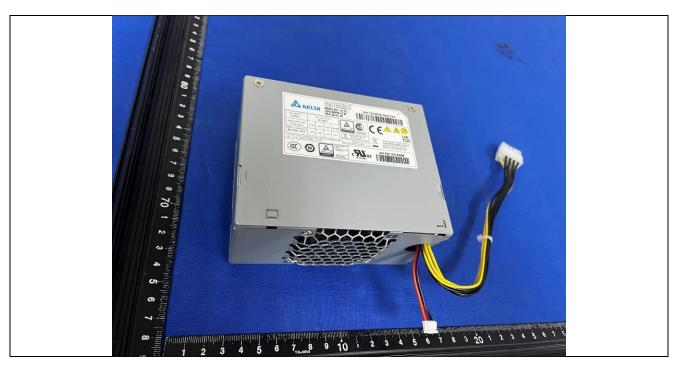
Details of: Built-in power supply (Model: DPS-80PB-10 B)
