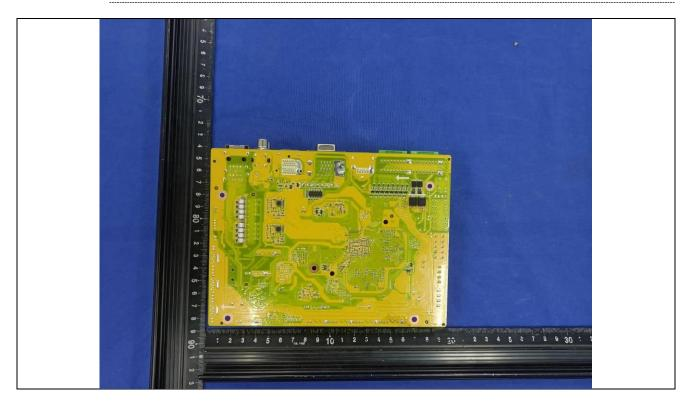
Details of: Built-in power supply (Model: SFXA1071A)
