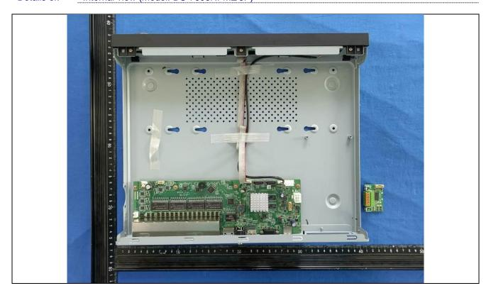
Details of: Internal view (Model: DS-7608NI-M2/8P)
