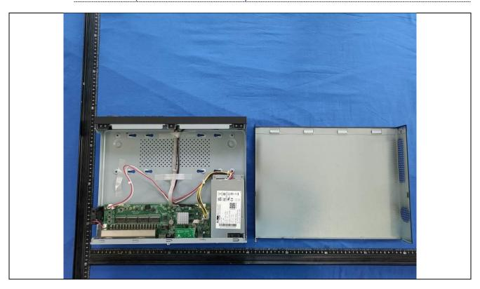
Details of: Internal view (Model: DS-7608NI-M2/8P)
