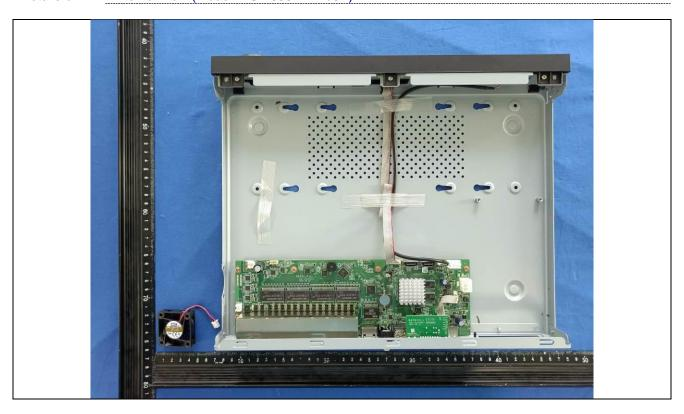
Details of: Internal view (Model: DS-7608NI-M2/8P)
