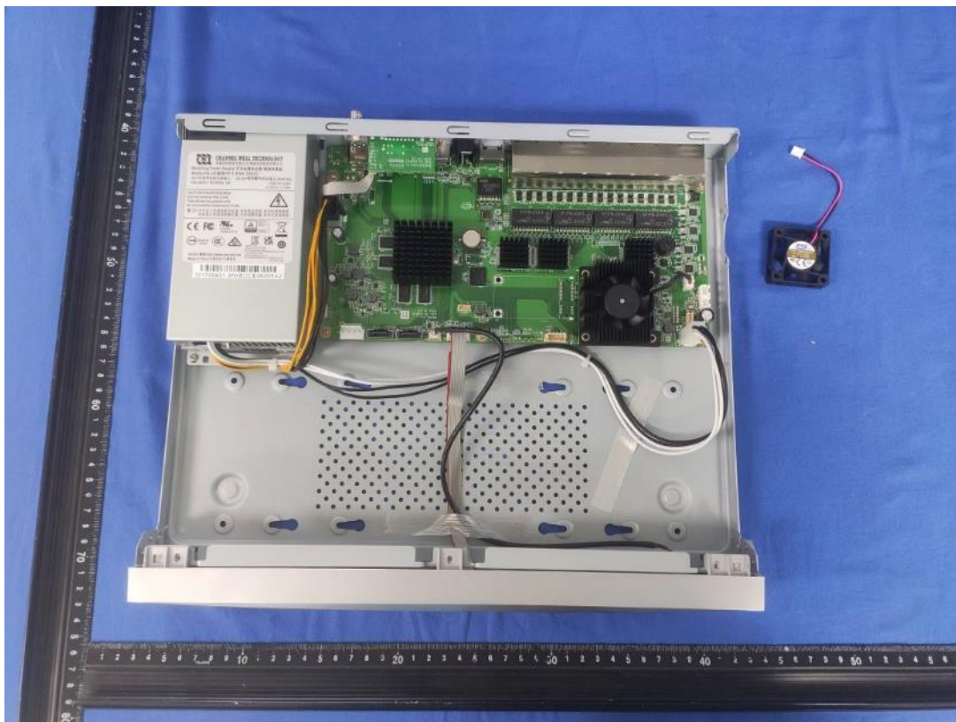
Picture 38 – internal view (include mainboard model: DS-80500)
