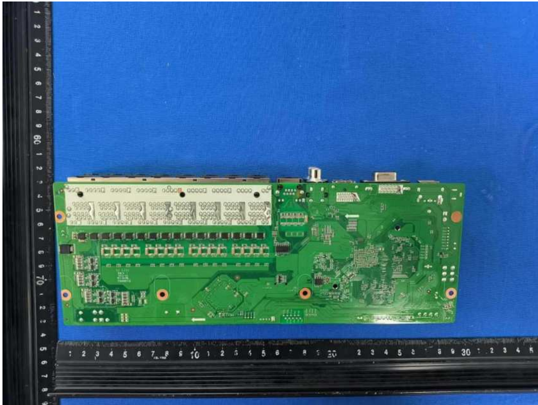
Picture 67 – PCB view (mainboard model: DS-80517)
