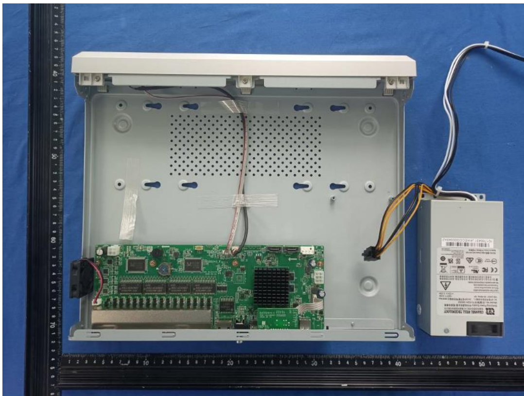
Picture 50 – internal view (include mainboard model: DS-80545)
