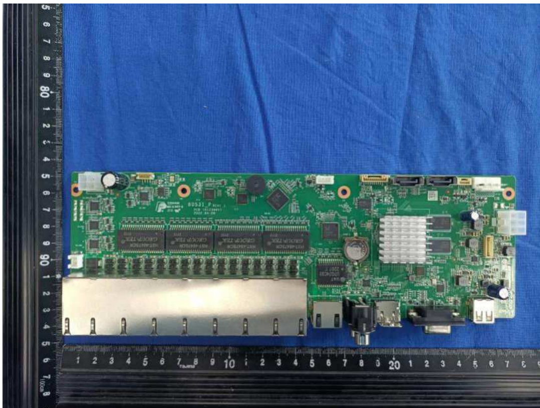
Picture 26 – PCB view (mainboard model: DS-80531)
