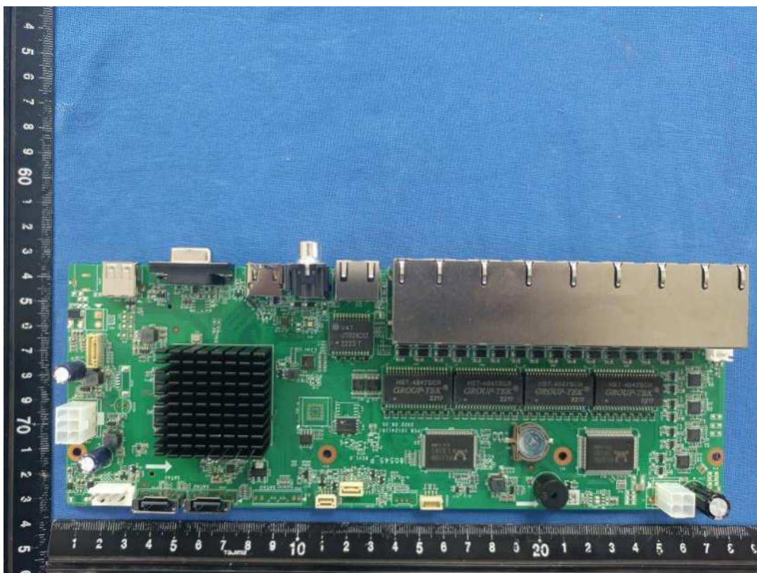
Picture 52 – PCB view (mainboard model: DS-80545)
