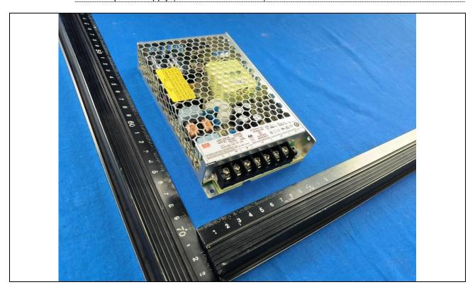
Internal power supply (Model: PMT-24V150W2BA) Details of:
