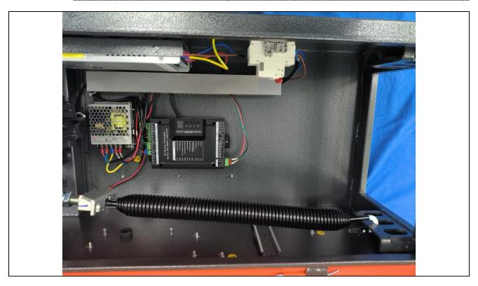
Details of: Alternative Building power supply (power for LED) PMT-12V50W2BA
