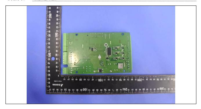
Details of: Building power supply (power for main board) (model: PMT-24V350W2BR)
