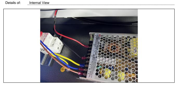
Details of: Building power supply (power for LED)
