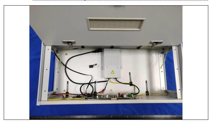
Details of: Internal view of Walk-through Metal Detector Case
