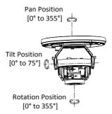
Figure 2-11 3-Axis Adjustment
