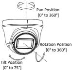
Figure 2-8 3-axis Adjustment
