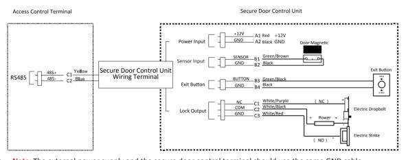
Note: The external power supply and the secure door control terminal should use the same GND cable
