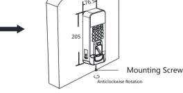
4. Tighten the screws to fix the terminal on the mounting plate and complete the installation.
