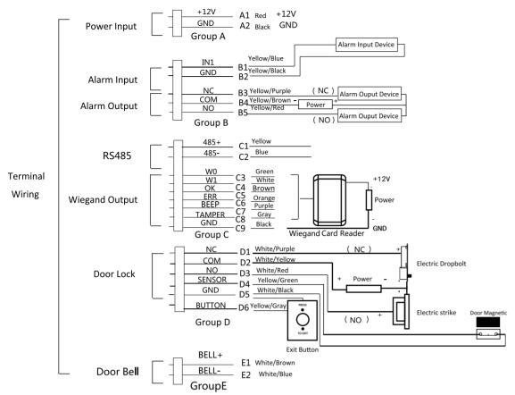
Note: The external power supply and the access control terminal should use the same GND cable.
