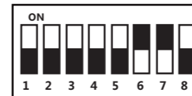
DIP Switch of Wiegand 26 Protocol
