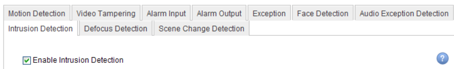
Figure 6. 12 Setting Intrusion Detection on IP Camera
