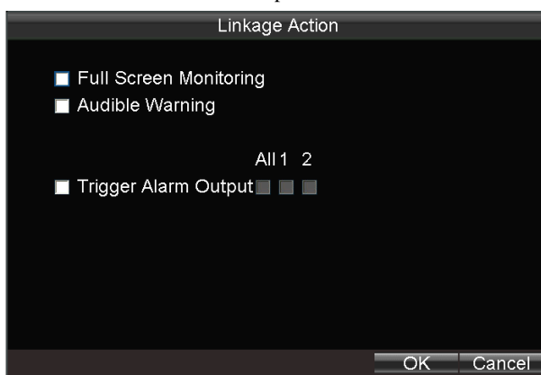
Figure 11.5 Alarm Linkage Action
