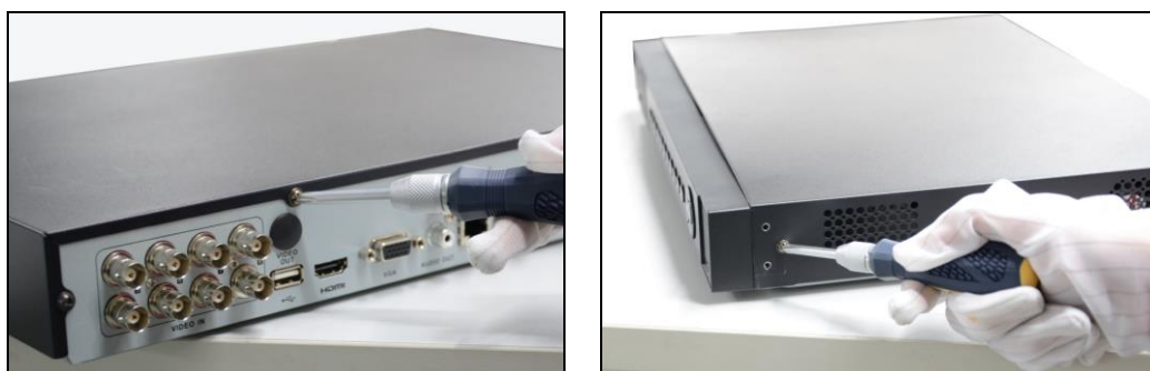
Figure 2-1 Fasten Hard Disk
