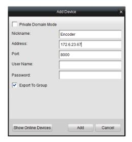
3. Edit a nickname for the device and input the IP address, port number (default: 8000), login user name (default: admin) and password (default: 12345) of the device.
