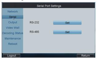
Figure 4.46 Serial Port Settings
