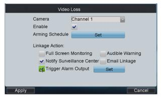
Figure 4.23 Set Video Loss Detection
