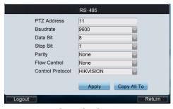
Figure 6.36 Set RS-485 Parameters
