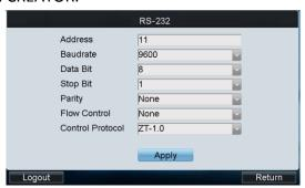
Figure 6.33 Set RS-232 Parameters
