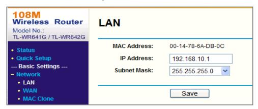
Figure A.2.2 Set the LAN parameters
