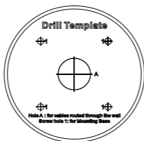
Figure 2-5 Drill Template of the Junction Box
