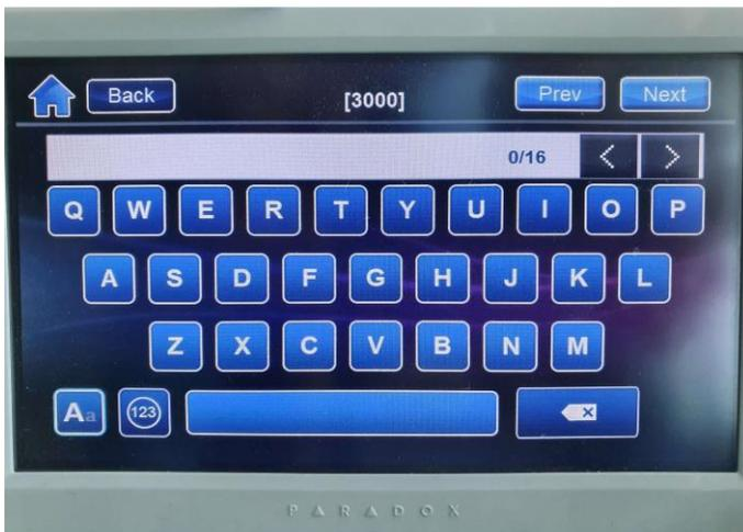
6) Once the code was received can be entered to keypad section 3000. Only TM50 and TM70 keypads can be used for entering codes as they support all (A-Z) characters contained by the license code.
