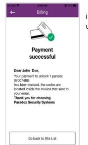
5) An email will be sent to the registered installer's email containing a PDF invoice. The invoice contains the unlock code(s), and instructions on how to unlock the panel's serial port for use with third-party devices.
