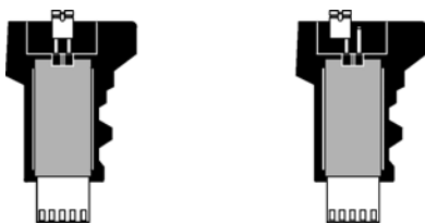
Figure 23: PMC-4 Jumper Settings Jumper On Jumper Off
