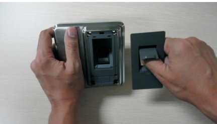
5) The plastic cover is being removed.
