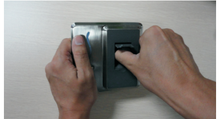
4) Remove the plastic cover on the device: The left hand holds the device, the right thumb stretches into the fingerprint sensor slot, the right forefinger press the right edge of the device. The right thumb pulls the plastic plate along the vertical direction to the device (the plastic plate is made of PC+ABS materials, with a strong anti-pull ability, will not be easily destroyed).
