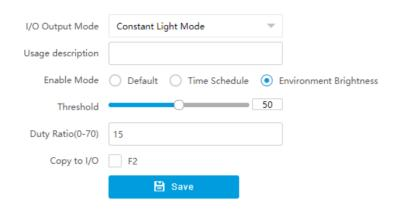
**Figure 3-2 Set Supplement Light Parameters**
