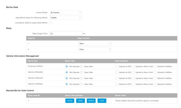
**Figure 3-11 Control Barrier Gate**
