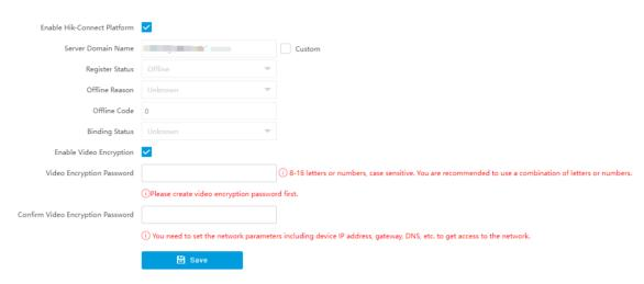
Figure 9-12 Connect to Hik-Connect (V3.0)
