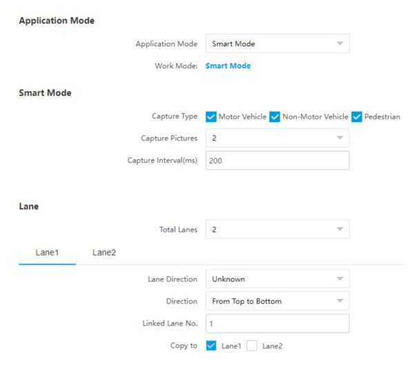
**Figure 2-1 Set Smart Monitoring Capture**
