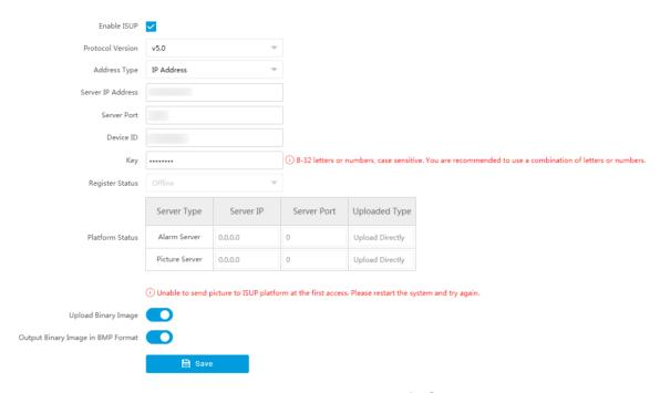
Figure 9-9 Connect to ISUP Platform
