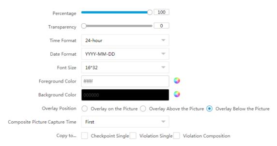
**Figure 3-6 Set Composite Picture Overlay**
