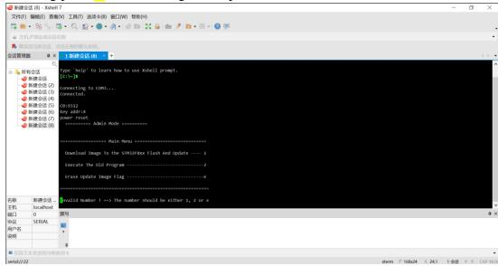
2) Press 1, CCCC will appear all the time, which means upgrade is possible.
