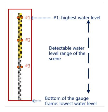
Figure 3-1 Adjust Calibration Lines and Gauge Range Frame
