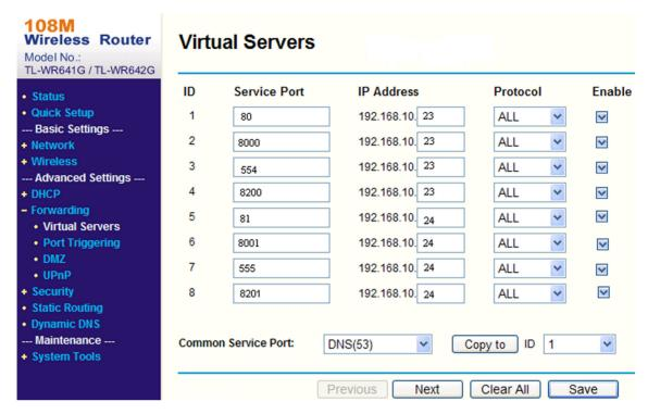
Figure 10-1 Port Mapping on Router
